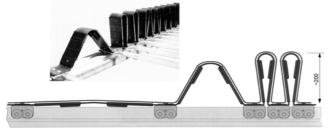
Patented frame construction enables easy and reliable tarpaulin roof opening and closing. The key element of this construction is multi layer rubber band that is capable for long term operating with numerous opening and closing. Center pillar rollers locks automatically when the pillars are fastened.
