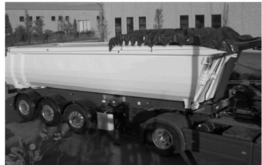
We deliver "EUROCOVER" tarpaulin system as a set of components. Mounting by the supplied instruction manual is easy and quick. Technical support is available and we can also arrange mounting and installation of complete system in the workshop of our subsidiary company.
