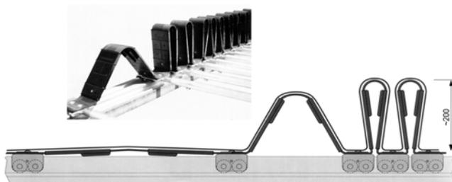
Patented frame construction enables easy and reliable tarpaulin roof opening and closing. The key element of this construction is multi layer rubber band that is capable for long term operating with numerous opening and closing. Center pillar rollers locks automatically when the pillars are fastened.
