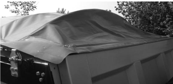
We adjust the length of the tarpaulin to the length of superstructure. The longest possible solution is 13500mm. Arch bearers insure that the tarpaulins remains in optimal shape. The arch height can be between 100 and 500mm as per customer request.
